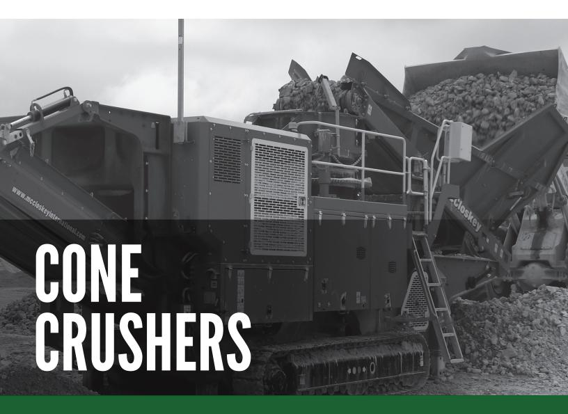
McCloskey mobile cone crushers have been designed to deliver superior performance whilst also achieving higher capacity, better product quality, optimum versatility, and improved fuel efficiency. Standard features are far from standard on McCloskey crushers, including an open chassis design, efficient conveyor design, recirc screen options as well as continuous load and material level monitoring.
